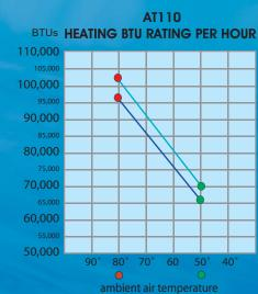
63% RELATIVE HUMIDITY / 80° WATER TEMPERATURE - RATED IN ACCORDANCE WITH ARI STANDARD 1160 80% RELATIVE HUMIDITY / 80° WATER TEMPERATURE - OUTSIDE THE SCOPE OF ARI STANDARD 1160
